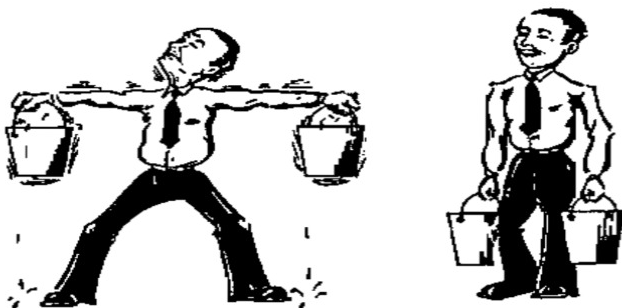
1,000 LB LOAD: 500 LB PER LEG AT 90°, 577 LB AT 60°, 707 LB AT 45°
